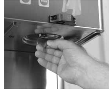
4. Insert the long end of sprayhead cleaning tool into the sprayhead fittings, and rotate several times to remove any mineral deposits from the fitting.
