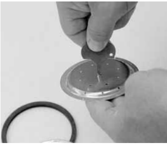
5. Use the pointed end of sprayhead cleaning tool to remove any mineral deposits from the sprayhead holes. The sprayhead holes must always remain open.
