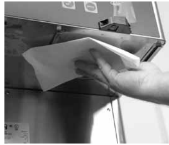
7. The use of a damp cloth rinsed in any mild, nonabrasive, liquid detergent is recommended for cleaning all surfaces on Bunn-O-Matic equipment. Do NOT clean this equipment with a water jet device.
