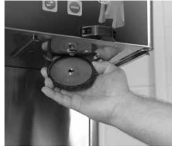
3. Remove sprayheads from brewer. Disassemble by removing the seal.
